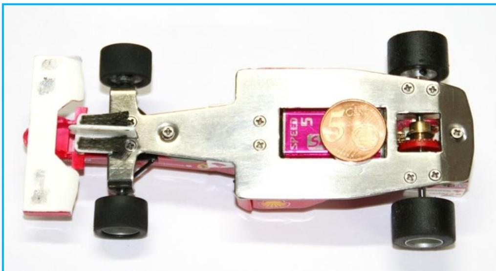
Width max. front axle with mounted tyres 62 mm
